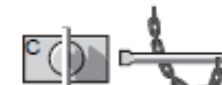
Chain interlock for large or poorly aligned sliding, hinge and lift off guards
